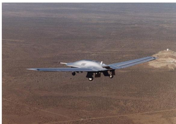
**Fig. 2: The DarkStar executing a fully autonomous flight in 1998 using the differential Global Positioning System. (Photo: Carla Thomas).**
