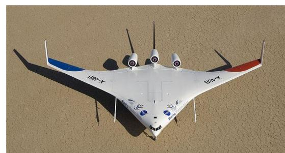
**Fig. 1: Boeing's X-48B Blended Wing Body technology demonstrator.**
