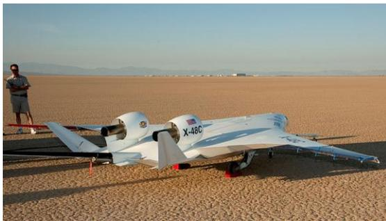
**Fig. 2: NASA-Boeing X-48C with inboard vertical stabilisers.** Photo: Carla Thomas.
